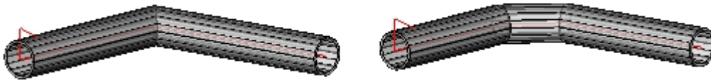
Before and after applying a chamfer on the axis of a profile
